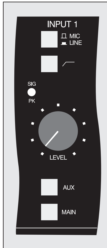
Figure 10. Detail of front panel showing mic/line input channel (typical of 3)
